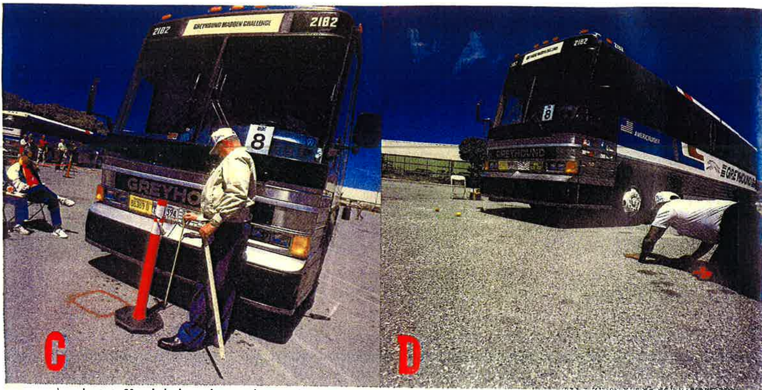
c) accelerate to 20 mph, brake, and stop within six inches of a pylon; and d) keep the bus' right-side wheels aligned between two rows of tennis balls.
